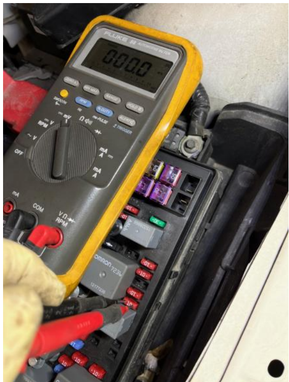
0.000mv Voltage Drop - No Current Draw on this Circuit
