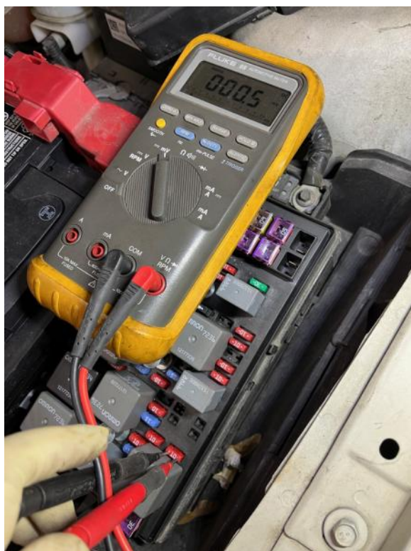
0.005mv Voltage Drop - There IS Current Draw on this Circuit
